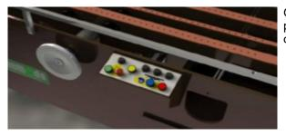
Operator controls are simple to understand and are premium quality ABB components. Quality in/Performance out. All 20" + VMC vacuum conveyors utilize operator adjustable vacuum modulation system(s).
