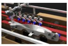
Plow Fold Kits attach quickly, adjustable tab smasher built into design. All sheet metal is stainless steel.
